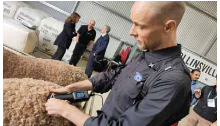
Ben Pullen of Woven Optics demonstrating the portable fibre micron testing device to IWTO Congress delegates on-farm at Collinsville Stud Merinos.
